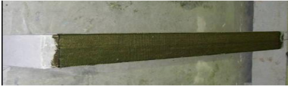
Figure 5: Beam strengthened with CFRP sheet for flexural (Group-1). (Nadeem A. Siddiqui 2009)
