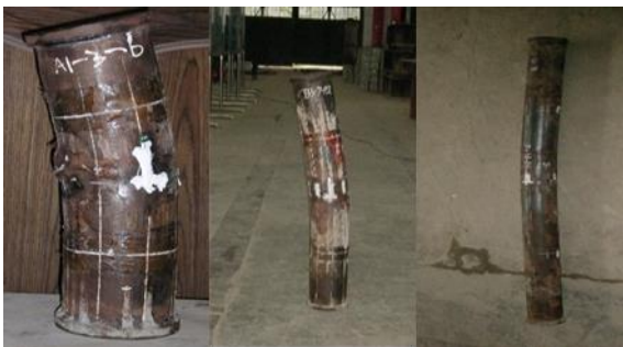
Figure 2: Typical failure modes of specimens
