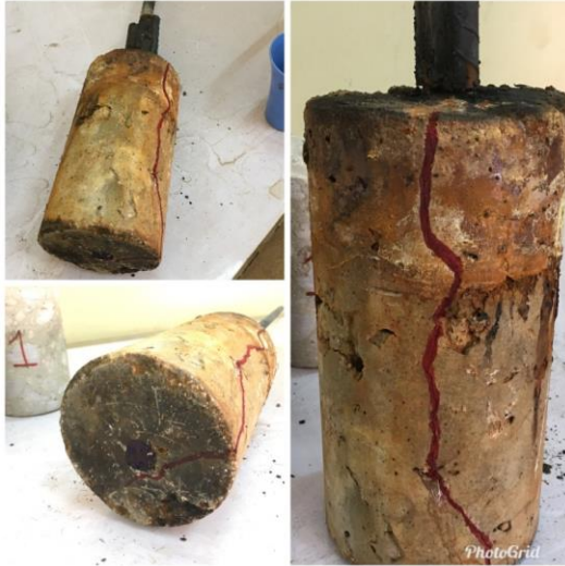
Figure 9: G 100-360 sample 3 Crack pattern
