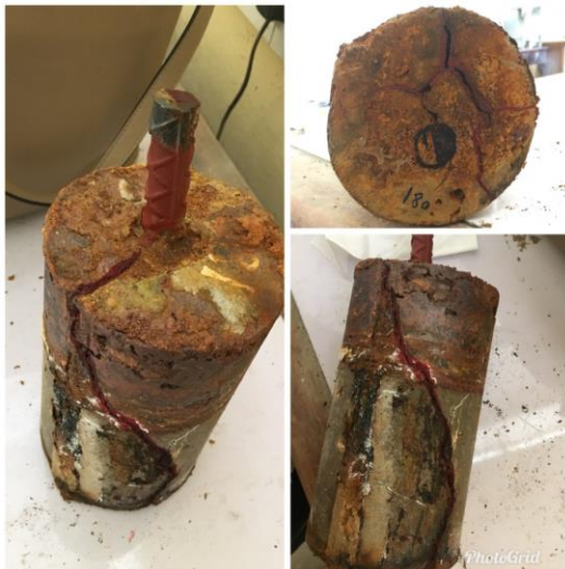
Figure 10: Crack pattern of G 100-180 sample
