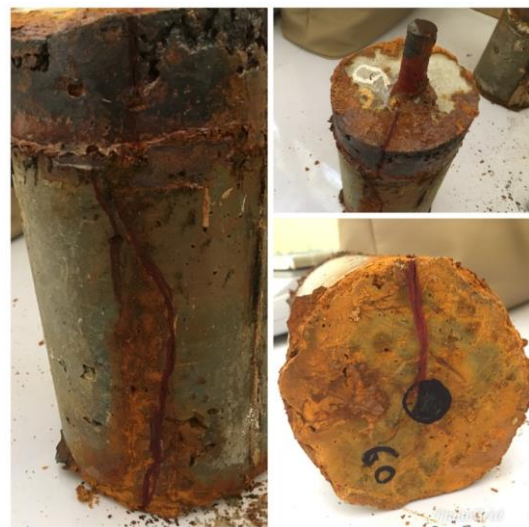
Figure 11: Crack pattern of G 100-60 sample
