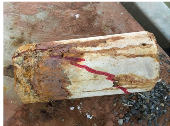
Figure 7: G 100-360 sample 1 Crack pattern
