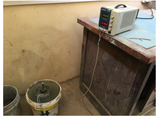
Figure 4: Accelerated corrosion test setup
