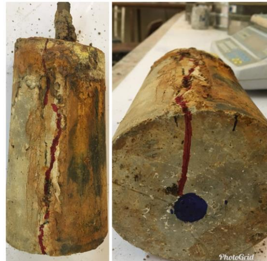
Figure 8: G 100-360 sample 2 Crack pattern
