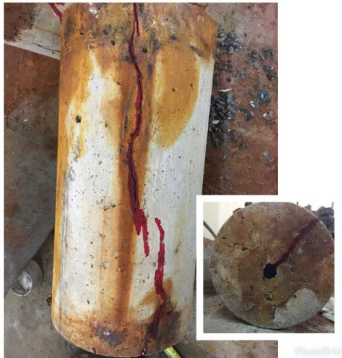
Figure 6: G 150-360 sample Crack pattern
