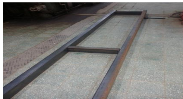
Figure3: Panel Pipe Framing
