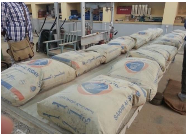
Figure 8: Panel 1 during Loading
