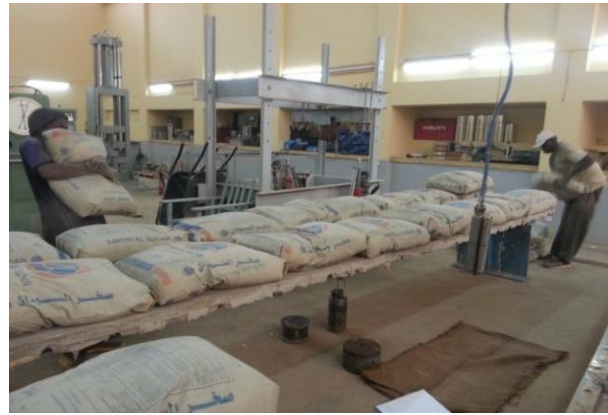
Figure 10: Panel 2 During Loading
