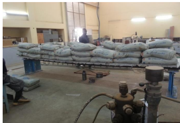
Figure 11: Panel 2 Full Loading
