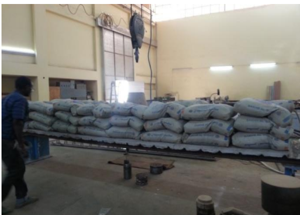
Figure 9: Panel 1 Full Loading
