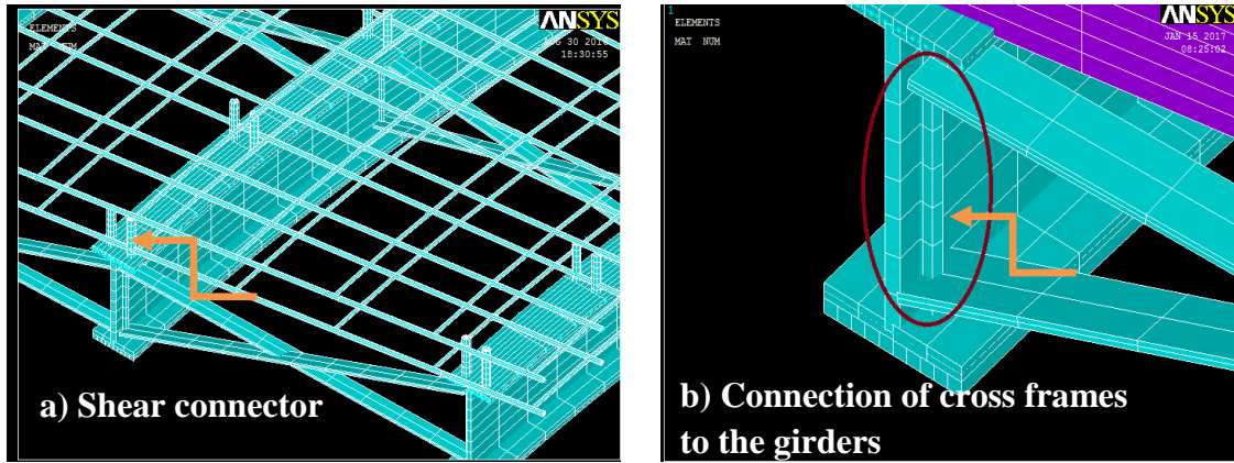
Figure 3: a) Shear connector on the top flanges, b) Cross frame fixation with the web
