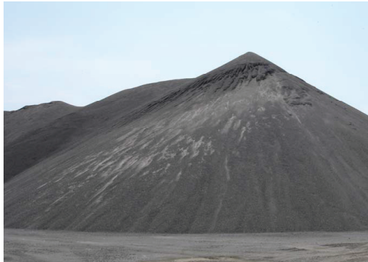
Fig. 2 Stockpiling of steel slag aggregates at crushing plant
