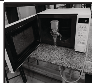
Figure 2. Microwave oven with the fit-in condenser and flat bottom flask
