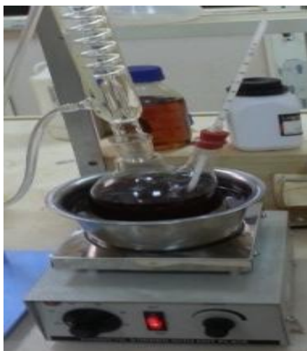
(a) Reaction of WCO with methoxide.
