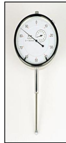
Fig. 2.a. Dial gauge with 0-50 mm travel
