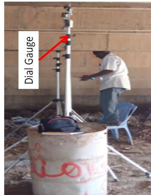
Fig. 2.b. Setup of three dial gauges for deflection measurement
