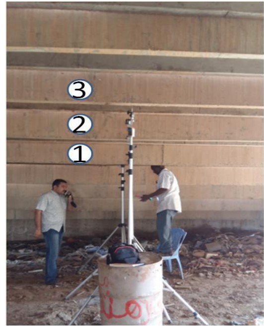
Fig. 5. Test beams and the setup of dial gauges
