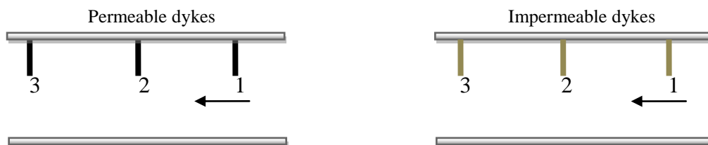
Fig. 5b. Arrangement of 3 spurs dykes (Flow depth=100 ,80 ,60,30,20mm)
