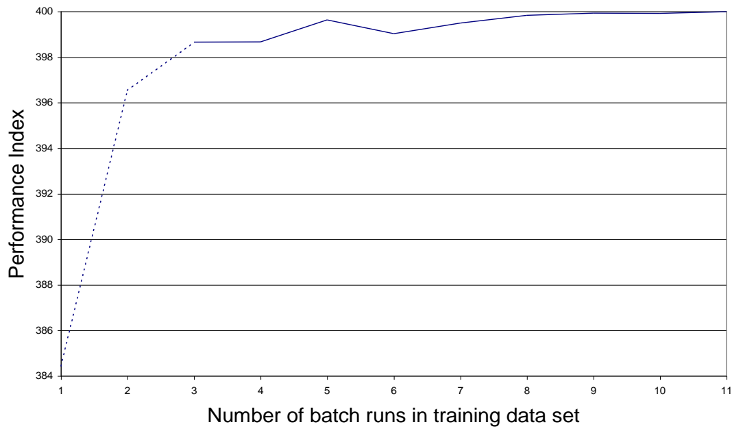
Figure (4). Incremental improvement in Performance Index with increase in number of batch runs for Case Study 2 (The dotted line refers to the Performance Index values of the 3 initial batch runs)
