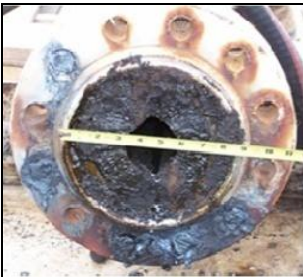
Fig (2). Flow line Clogged by Scale
