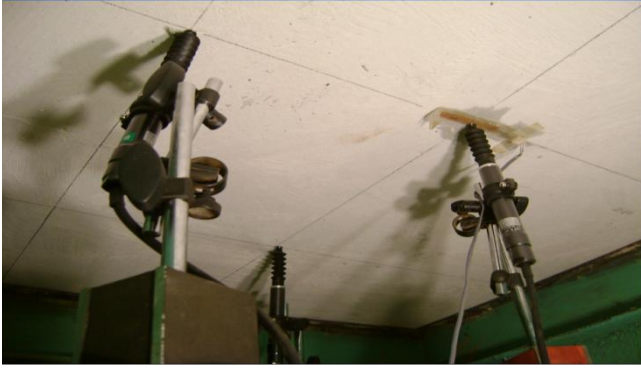
Fig (4). Location of deflection measuring points and Strain gauge and at the bottom of slab
