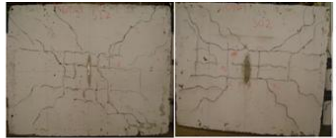
(a) (b) Fig (11). Slab (a) SI2 and (b) SO2 after failure
