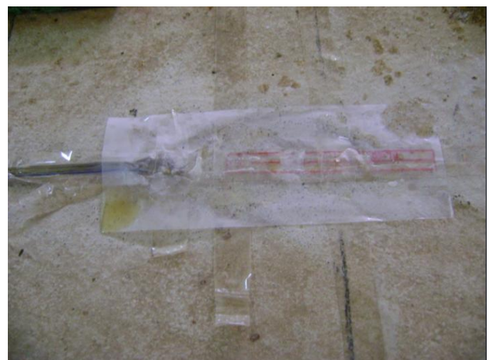
Fig (3). Typically installed strain gages on the top concrete specimens.
