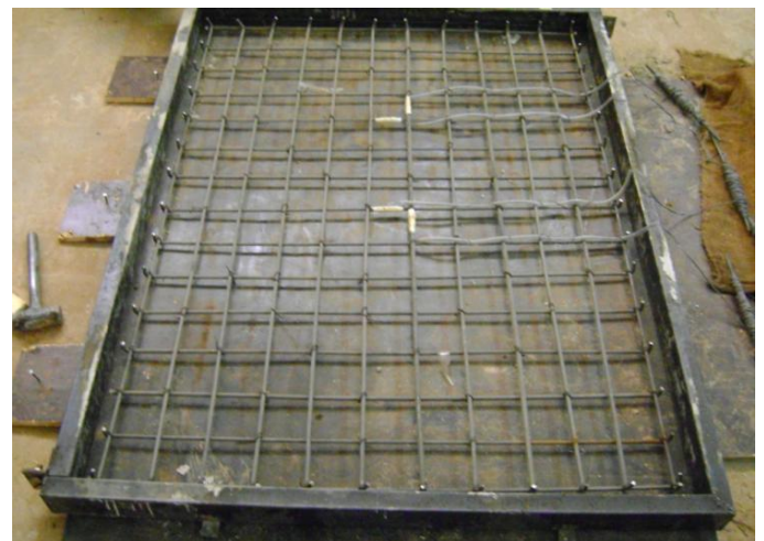
Fig (2). Typically installed strain gages on the bottom reinforcing bars.
