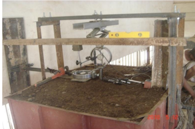
Figure (2). Test setup and loading arrangements for vertical and lateral loading
