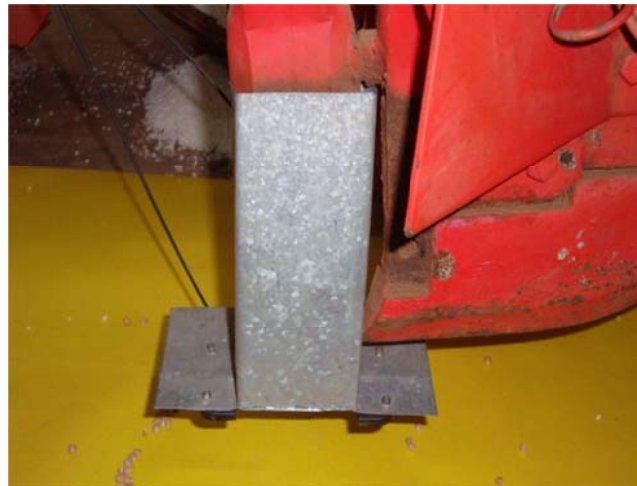
Figure (5). The Fiber Head connected to the seed tube
