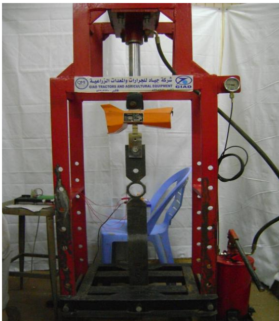
Figure (7). Calibration setup of drawbar transducer
