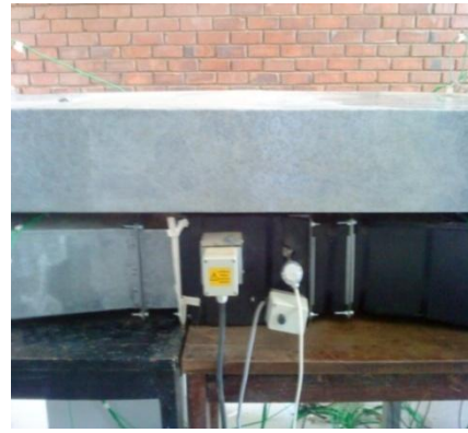
Figure (3). the electric heater
