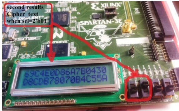
Fig.19: The second output Cipher text result when sel=2'01
