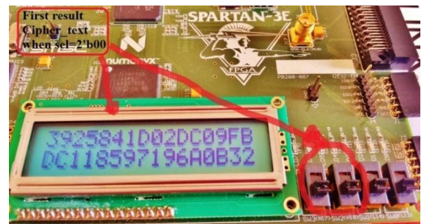
Fig.18: The first output Cipher text result when sel=2'b00
