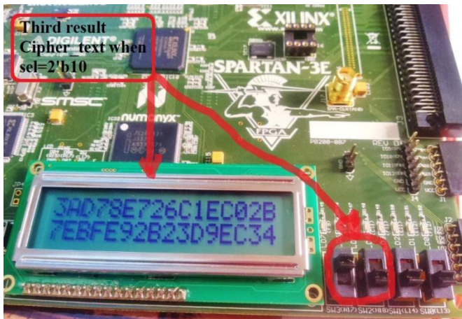
Fig.20: The third output Cipher text result when sel=2'10
