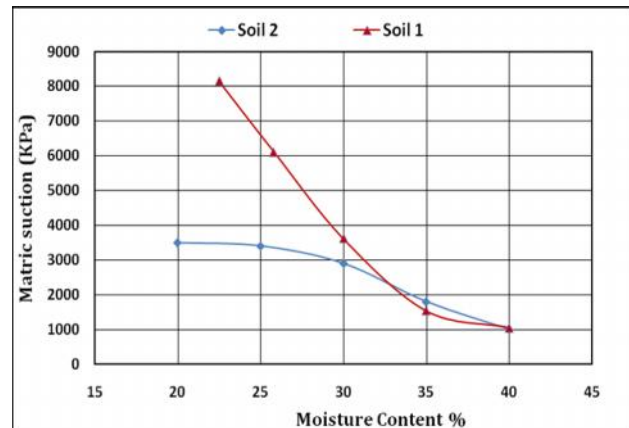
Fig. 1. Soil water characteristic curve for Soil 1 and Soil 2
