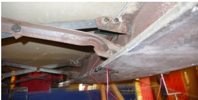
Fig.20. Torsion of exterior girder and buckling in middle cross frame for full interaction curved specimen
