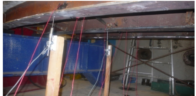
Fig.14. Curved model Instrumentations-LVDT to Meager Girders Deflections
