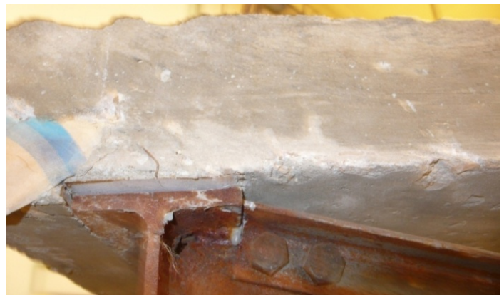
Fig.22. Slip in mm at exterior girder after static test of curved partial interaction specimen
