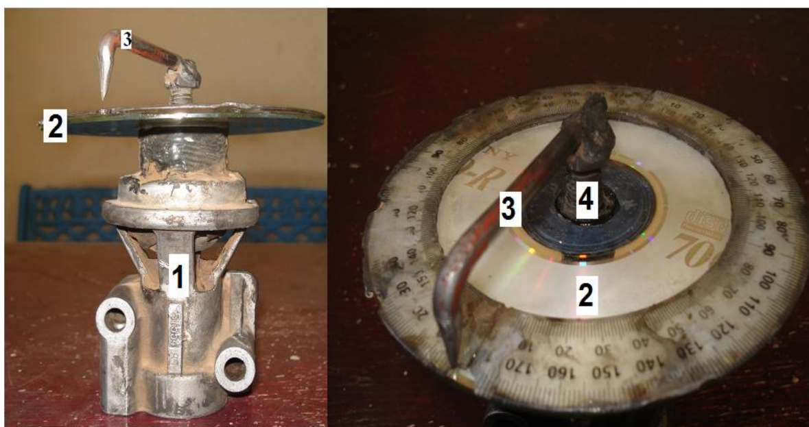
Fig. 1. EGR valve. 1- EGR valve. 2 – 360deg. Protractor. 3 – Pointer. 4- Rotating bolt
