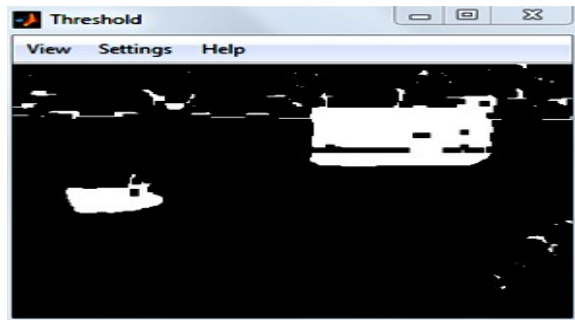
Fig. 7. Video Frame After Autothresholding.
