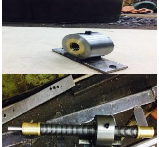
Fig.7. LEAD SCREW and nut Assembly
