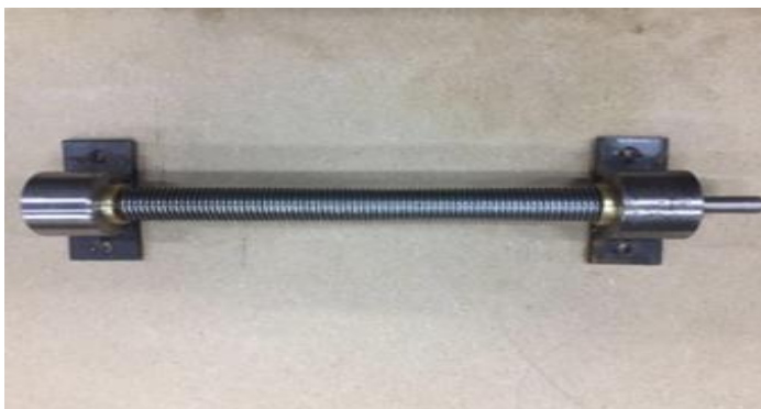
Fig.6. LEAD SCREW and BEARING Assembly
