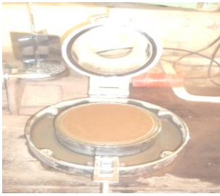
Fig.3: Sheet forming on the bottom screen
