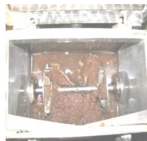
(h): Mixer rotates for 5 min.
