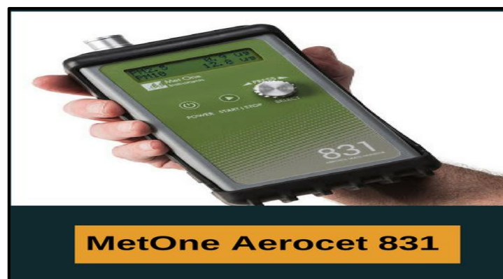
Fig. 2. Device for measuring particular matter (Aerocet)
