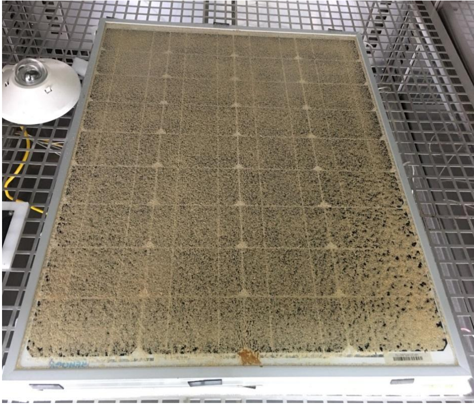
Fig. 2. Photographic view of PV module inside the chamber with 59g of plaster soil uniformly distributed on its top
