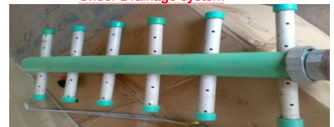
Fig. 7. Design of under-drainage system (dimensions in cm)
