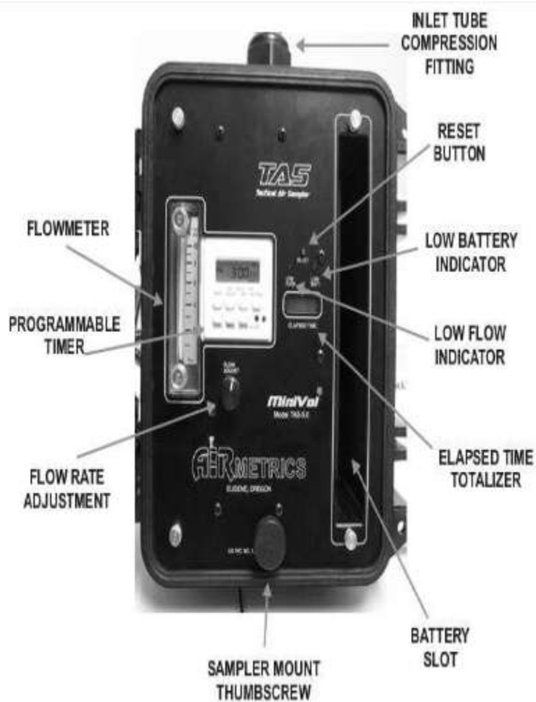
Fig. 4: MiniVol air sampler layout
