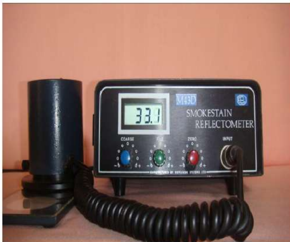
Fig. 5: The Smoke Stain Reflectometer that was used for measurement of the black carbon.
