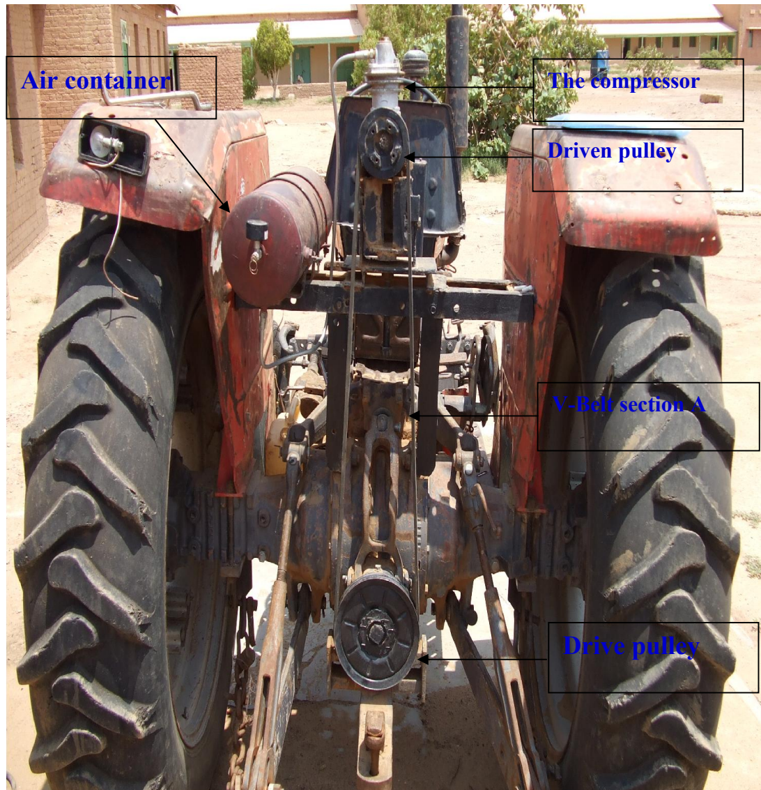
Plate 1. Parts of the designed air compressor installed on the rear of tractor
