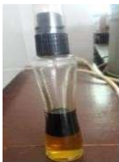
Figure 7. Liquid oil obtained as the final product after thermal cracking. (Source: Authors' experiment, 2017).
