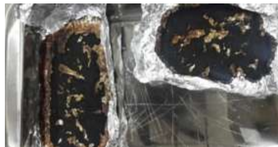
Figure 1. Final bioplastic product obtained using the initial approach. (Source: Authors' experiment)
