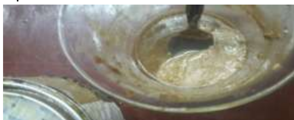
Figure 3. Self-separation of the mixture and formation of bioplastics. (Source: Authors' experiment) separated bioplastic material was then transferred into a Petri dish and dried in an oven at 60 °C until a constant mass was achieved, as shown Figure 4.
