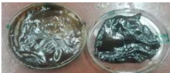
Figure 4. Final bioplastic product obtained from banana peels. (Source: Authors' experiment)
