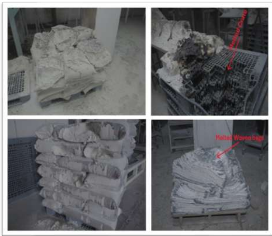
Figure A .5: Melted crates and wheat woven bags without flour ignition [25]
